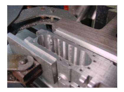
Using the same 0.750" diameter mill, follow the limits below for a second roughing pass. The numbers are caculated to leave 0.005" for final clean-up.
