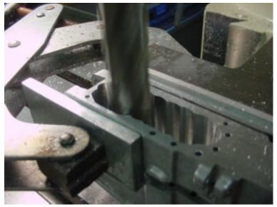
Now with a 3/4" diameter end mill (3" long) rough plunge out the material along the centerline. It is best to take out as much as possible with a heavy end mill so the smaller one will be under less stress. The dimensions shown below are the limits for this operation. The plunge positions inbetween are not critical. Take the first plunge on center of one of the inner 1/2" holes. Then move approximatly .3" for each successive pluge, but be careful not to exceed the limits.
